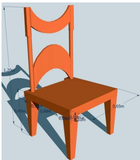
Figure 11.a,b. Sketchup® 3D representation of the marble chair represented in the Cycladic statuette from Naxos island (Naxos Museum), illustrating the suggested dimensions (left) and joints (right) of the actual wooden construction (Tsiptotas, 2010)
