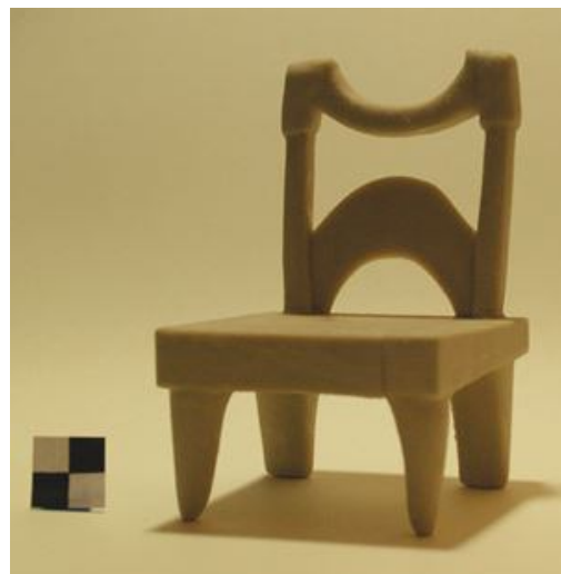
Figure 15.a,b. Final printed model of the marble chair represented in the Cycladic statuette from Naxos Island (Naxos Museum), created by 3DS Max® and printed by Zcorporation Zprinter® 450
